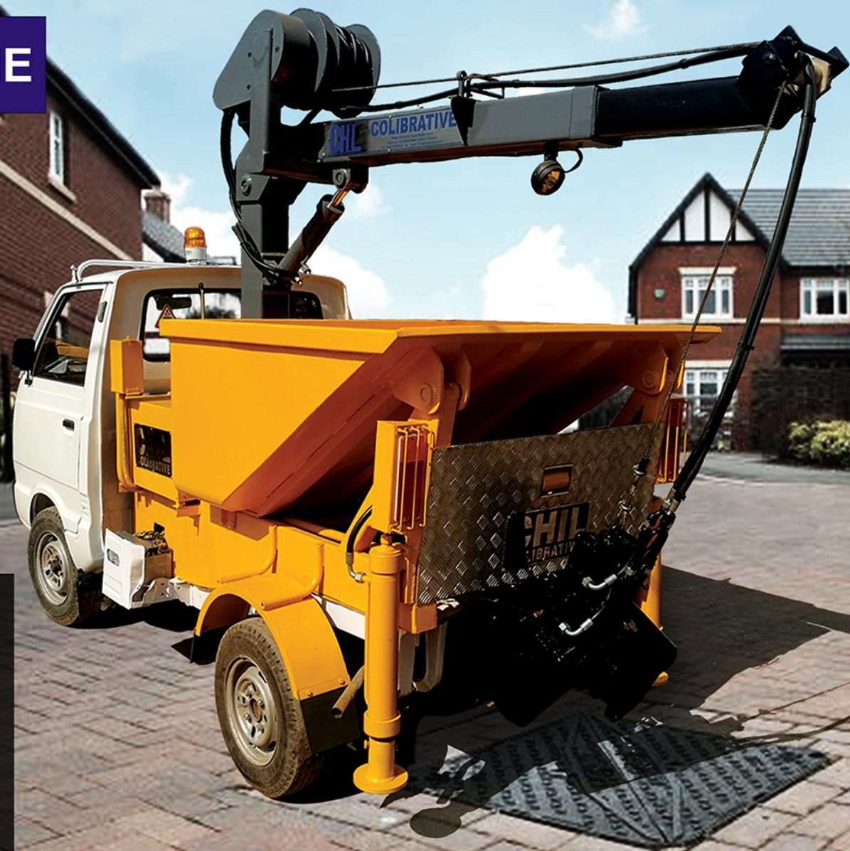
CHIL Desilting Machine is an original CHIL Design, specifically engineered to cater Pakistan's need of cleaning deep manholes. The vehicle is able to operate upto 50 feet deep and in manholes with diameters as small as 1.5 feet. This allows for a quick and effective solution to sewer blockages under the most hazardous conditions, providing a comfortable and healthy life for citizens of the locality.
